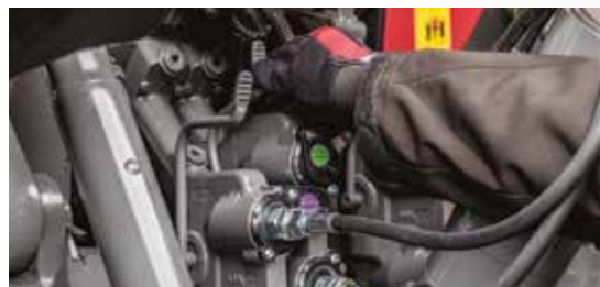
Conveniently located decompression levers
